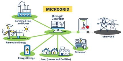
this bill is microgrids based on a self-sourced generation of a minimum of 20 Megawatts (MW). A graphic from the federal Department of Energy (See footnote 1) illustrates the idea. The microgrid is capable of being independent of the grid but can also sell surplus power to the grid.
